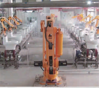
卫浴喷釉集成生产线 Application of glaze spraying shop for sanitary ware industry
